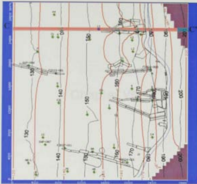
Fig. 48. Observed versus simulated water level elevations in the upper aquifer for the 2010 prediction simulation, Al Wagan area, UAE.
